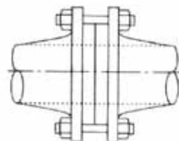
Stub End with Steel Backing Flange
