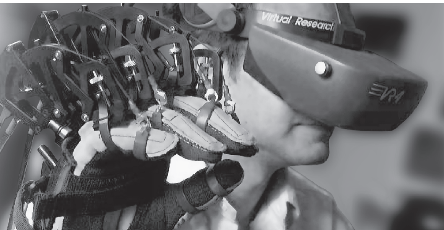
▲ Figure 2: Addition of haptic device on VR user's hand to allow for "touch sensation"
